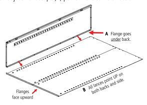
**4.** Attach the top (Ref. No. 5) to the unit by sliding the outer flange over the back of the unit and the side flange on
