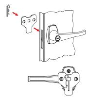
**3.** With the handle still in the open position, hook the locking bars (Ref. No. 13) to the locking cam (see "A" at left). Once in position, slowly rotate the door handle to the closed position so the lock bars prot rude from the holes at the top and bottom
