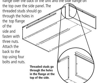
**5.** Attach the right side (Ref. No. 3) to the back in the same manner as you did in step 3, again, making sure that the flange is around the back and that the lances on the shelf adjustment strips are pointed in the same direction as those on the back and left side. Push the side panel up so the studs in the top go through the holes in the top
